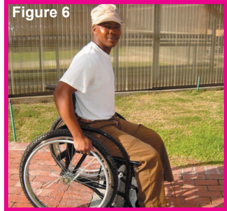
Figure 5 & 6: The longer wheelbases of the rural WORLDMADE 3 (Shonaquip) and the dual purpose ROUGHRIDER (CE Mobility), allows the user to access very steep gradients with safety
