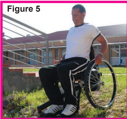
Figure 5 & 6: The longer wheelbases of the rural WORLDMADE 3 (Shonaquip) and the dual purpose ROUGHRIDER (CE Mobility), allows the user to access very steep gradients with safety
