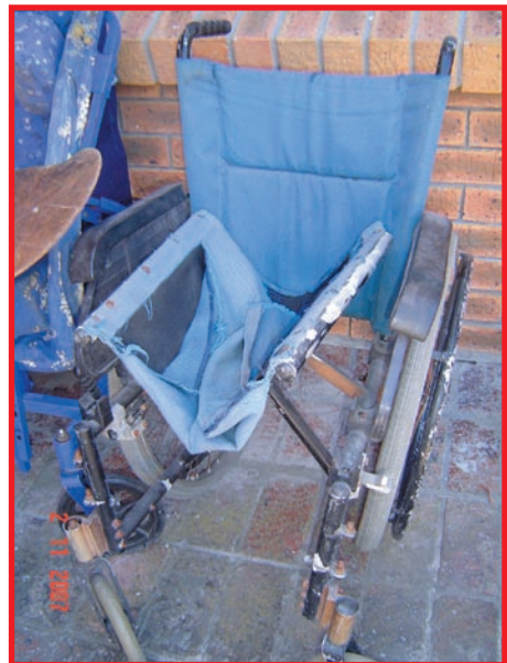
Figure 22: Cracked frame, torn upholstery and bent cross-bars after a short period of use by an active user
